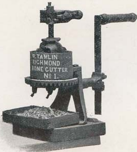
No. 1.—Weight 37 lbs. Capacity, 10 to 12 lbs. per hour. Diameter of Hopper, 6 ins. Telegraph Depth of Hopper, 4 ins. Code, “Rose.” Price, £1 8s. Od., carriage paid.
