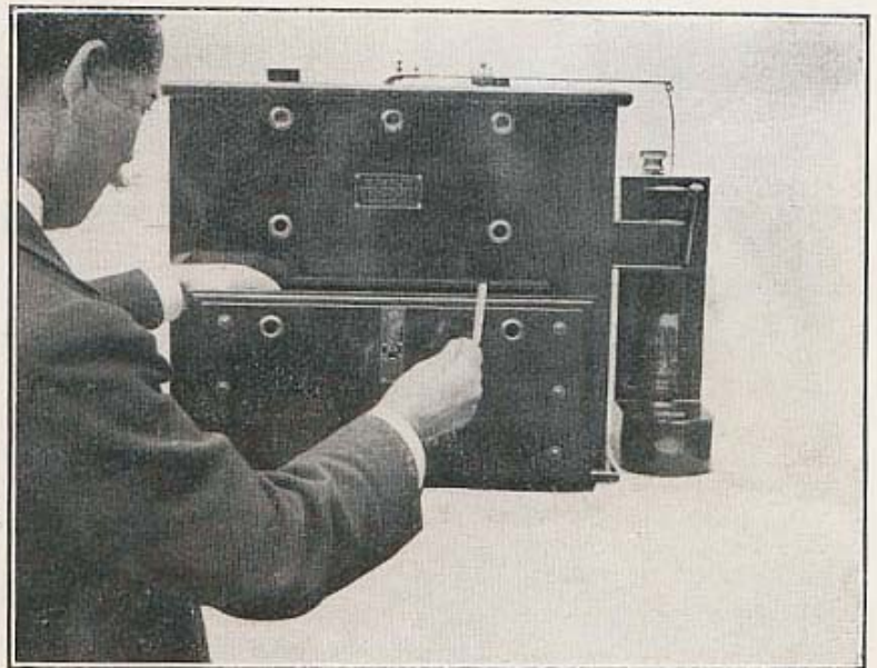
SHOWING METHOD OF PUTTING IN THERMOMETER.
